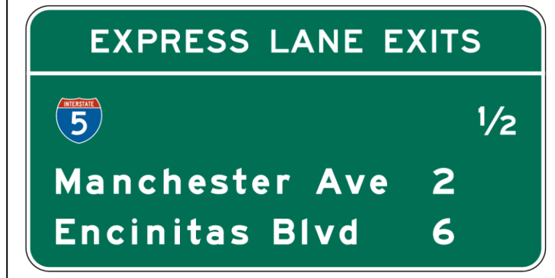
Figure 2G-19. Example of an Exit Destination Sign for a Managed Lane
