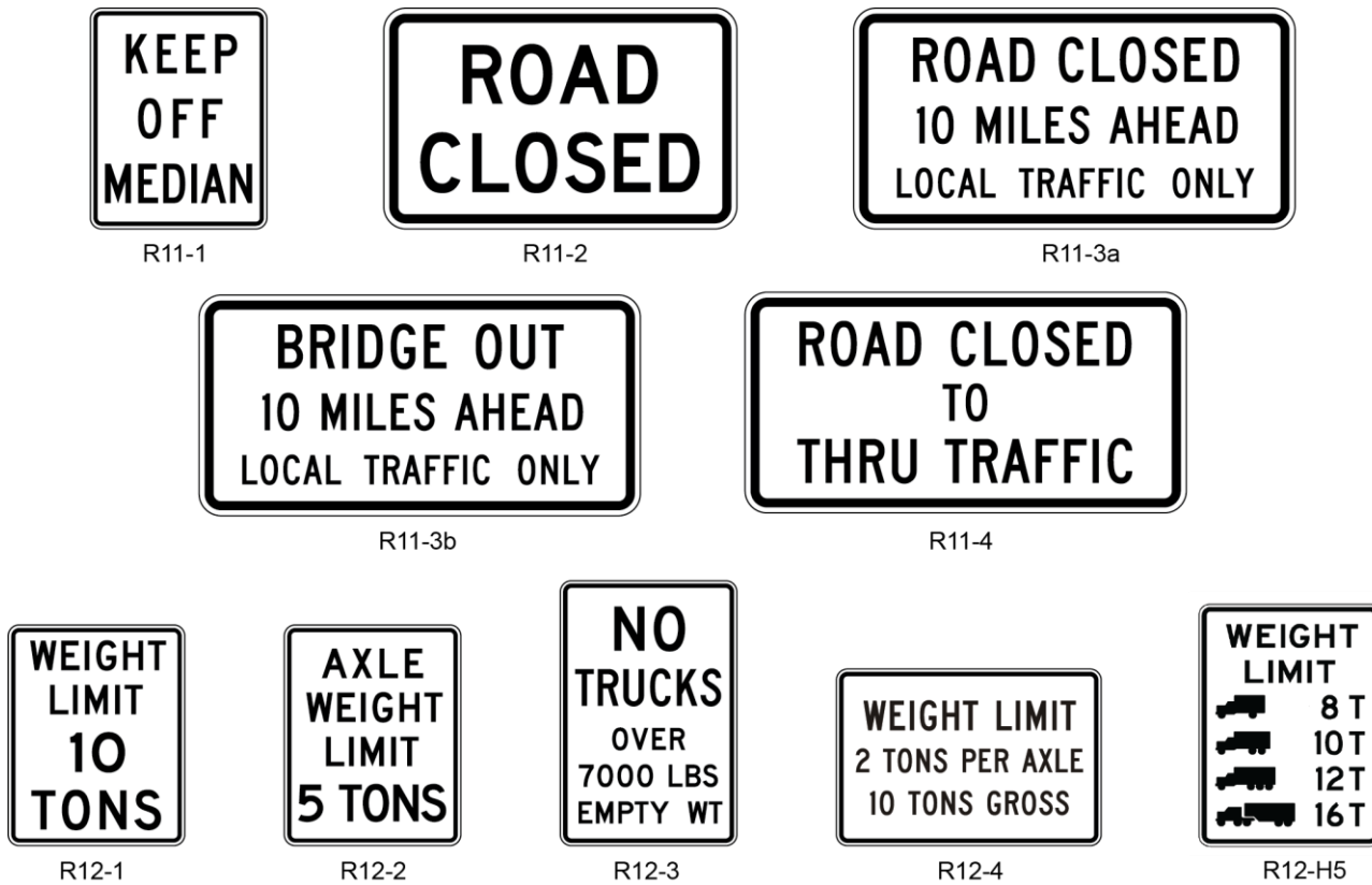
Figure 2B-29. Road Closed and Weight Limit Signs
