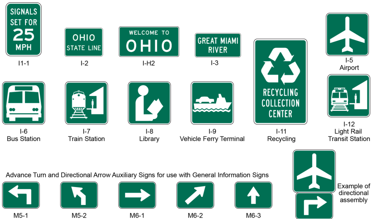
Figure 2H-1. General Information and Miscellaneous Information Signs
